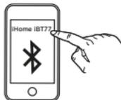
3. To pair with a different device or at a different time, make sure unit is powered on, then *press and hold* the **Bluetooth/Speakerphone/Play/Pause Button** for 2 seconds. Select “iHome iBT77” on device to pair.
