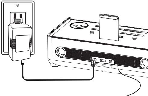
Attach AC adaptor cable to DC jack on back of the unit and plug the other end into a wall socket. Remove pull tab from the backup battery compartment on the bottom of the unit. Extend FM antenna for best reception.
