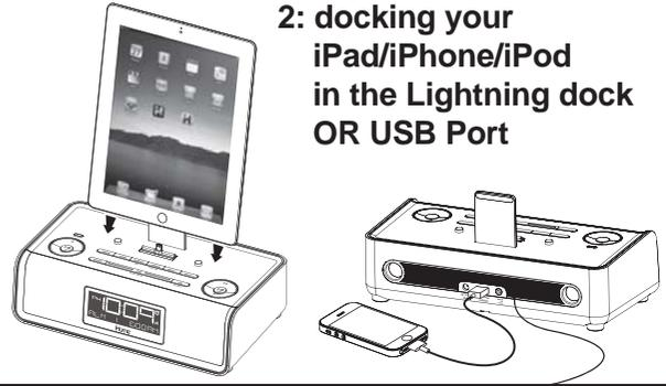
While the dock accommodates most cases, you may need to remove your case for proper docking. Gently dock any iPad, iPhone or iPod with Lightning connector onto the Lightning dock on top of the unit. The device will charge while docked. Press the **▶ Dock Button** on the unit to play your iPad/iPhone/iPod. Connect an iPad, iPhone or iPod to the USB Port on the back of unit using the connecting cable that came with it to charge and play (press the **▶ USB Button**).
