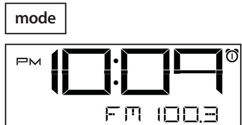
Press and release the **Mode Button** as needed to select FM band. Press and release the **+ or – Button** to tune in a station. See page 5 for programming presets.
