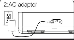
Plug the AC adaptor into the DC jack on the rear of the iP46 and the other end into a working outlet. The internal battery will charge.
