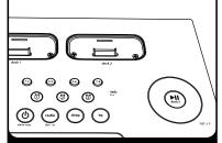
Press the Radio button and turn the Set Wheel to tune in a station. See page 4 for programming presets.
